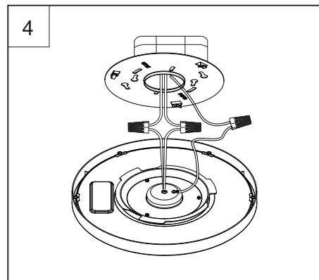
Step 4: Making the Wiring Connections.
