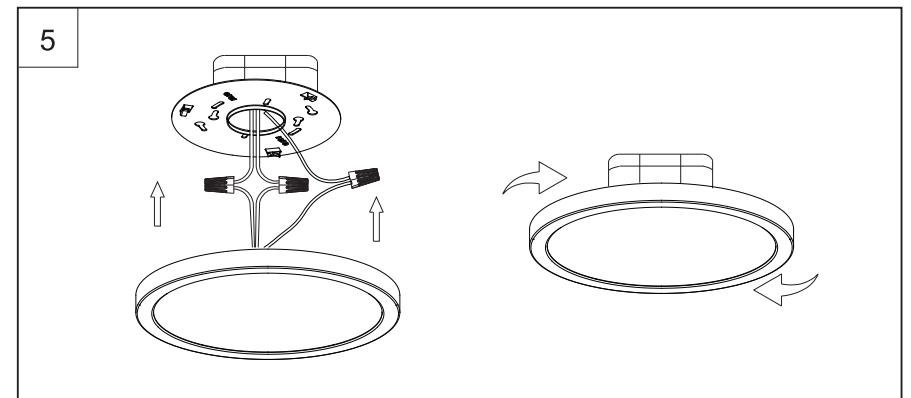
Step 5: Attaching the LED fixture to the Junction Box.
