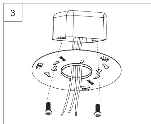
Step 3: Installing the Mounting Plate.
